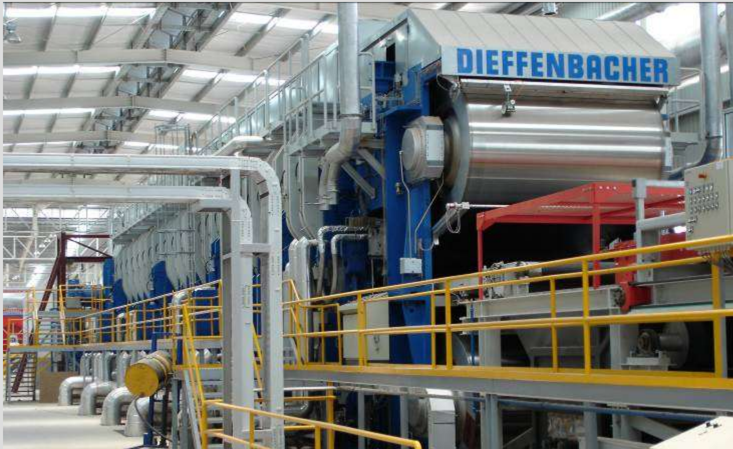
Line for the manufacture of wood based panels
