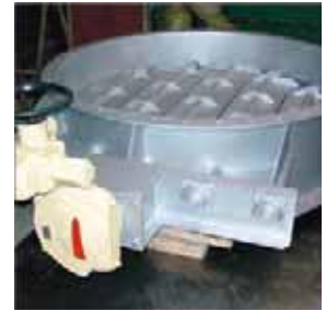
Control flaps for flue gas and ambient air
