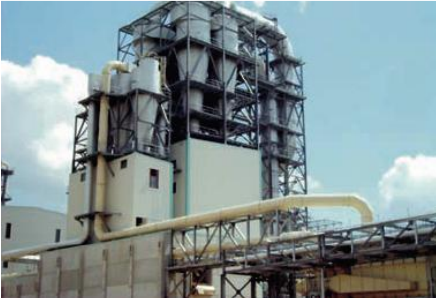
FTU Single stage fiber dryer with re-circulation system
