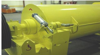
PLC controlled discharge flap
