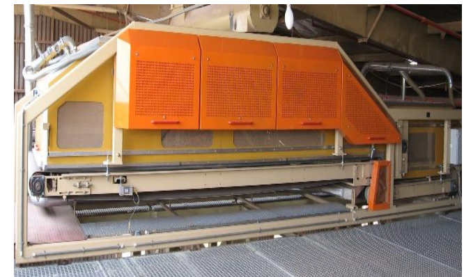
Flake dosing bins are equipped with reliable load cell measurement system.
