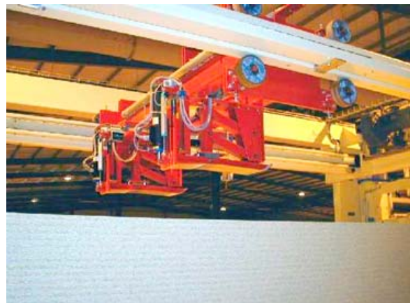
Feeding pusher feeds the topmost board of the stack. The feeding nails adjust automatically according to panel thickness.
