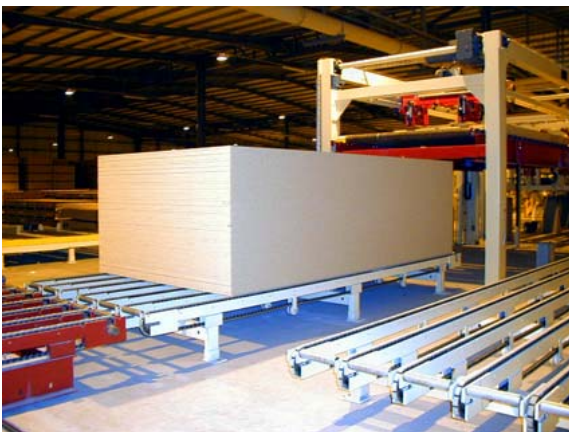
Chain conveyor takes the stacks to feeding station
