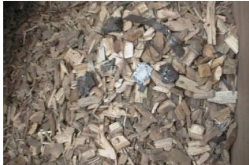
Separated heavy particles like stones etc.
