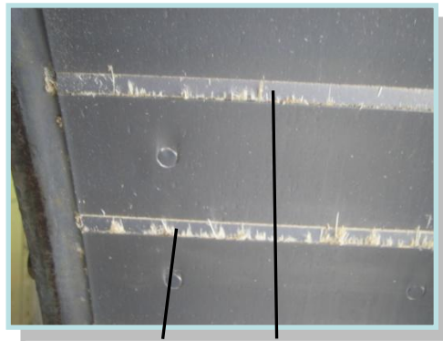
Cutting edges of knives covered by soft wood fibres
