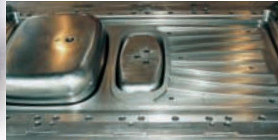
2nd draw tool for the manufacture of a 1 1/2 bowl sink
