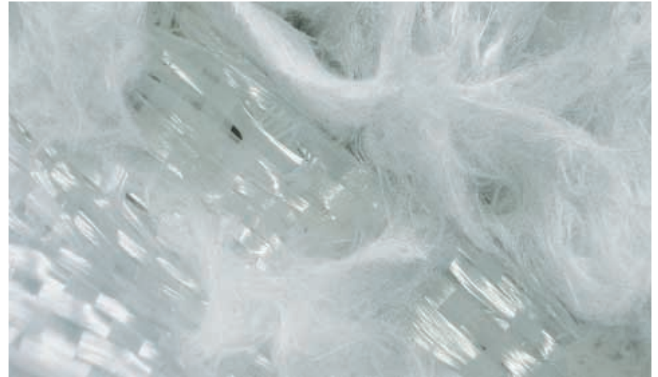
Incinerated compression part segment – The long fibers have penetrated the endless fibers and filled the rip structure. The endless fibers have kept their position and hardly been damaged by this penetration.
