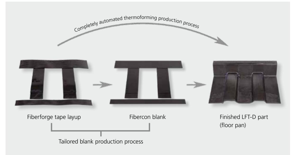
High-volume production of tailored fiber reinforced thermoplastic composites
