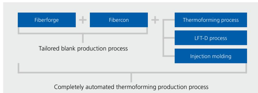
Using Fiberforge and Fibercon together with downstream systems, such as the handling robot and forming press, more than one million parts can be manufactured per year on just one line. As system supplier of this production line, Dieffenbacher is able to ensure a smooth process and optimum system availability.
